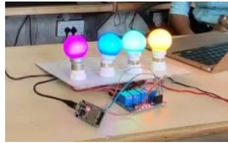
Fig. 8 Operating 4 Bulb via Bluetooth Application
